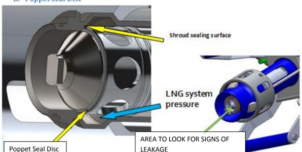
When the poppet seal disc is worn or damaged the leakage can be detected **ONLY** when nozzle is decoupled from the receptacle and pressurized.
