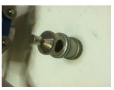
• If Phillips screw is installed as shown, use Phillips screwdriver to remove it. Otherwise, use 5/32" hex Allen wrench.
