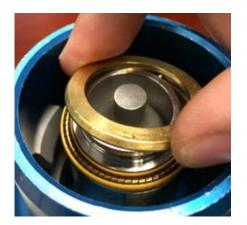
• Remove used Spring Energized Seal (B78705-6)
