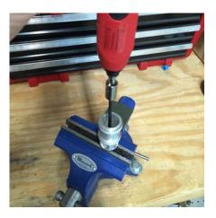
• Clean off excess Anti-Seize Compound from the Poppet Assembly and reinstall back into the nozzle.
