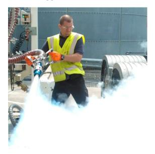
Sometimes leakage can occur due to the poppet not closing off LNG supply. Visual appearance of the escaping LNG could range from a mist to full exposure of gases; this depends on the rate of pressure and the position of the poppet.
