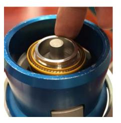
Carefully install new Spring Energized Seal (B78705 6)
