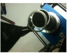
• Remove Tube Spacer (P/N B84399-1)
