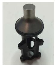
• Hold nosepiece in bench vise and use 5/32" hex Allen wrench to remove screw.
