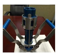
Remove Retaining ring (B91877SS-112) using Retaining Ring Pliers
