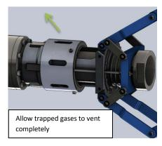
When venting is completed, pull handles fully towards the operator to remove the nozzle from receptacle.
