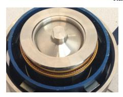
• Remove used Nozzle Seal (93209)
