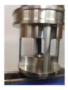
• Clean off excess Anti-Seize Compound from the Poppet Assembly and reinstall back into the nozzle.
