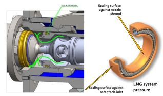
surfaces creating a tight barrier to prevent gas or fluids from leaking. The spring also provides resiliency to compensate for seal wear, gland misalignment or eccentricity. While spring force provides adequate force for sealing at low pressure, at high pressure the system pressure augments the spring force to provide an even tighter seal.
