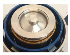
• Remove used Nozzle Seal (93209)
