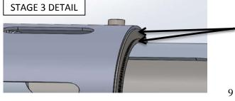
Pull handles until the plate stops at retaining ring
