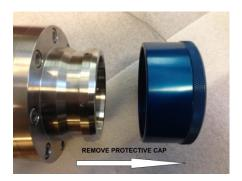
Thoroughly clean nozzle and receptacle connections with dry compressed air or nitrogen. Ensure that no dirt or ice is visible on either the nozzle or receptacle.
