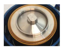
• Carefully install new Nozzle Seal (93209)
