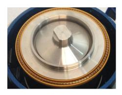
• Carefully install new Nozzle Seal (93209)
