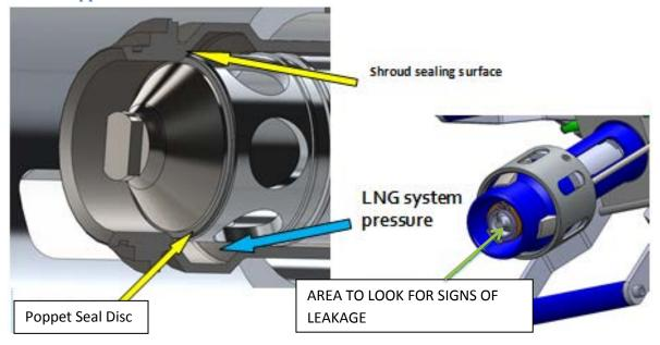
When the poppet seals are worn or damaged the leakage can be detected **ONLY** when nozzle is decoupled from the receptacle and pressurized.
